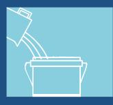
Add 400ml of GRESBOND Premium Grout Admix KGA-01 in 1 kg grout and mix until a slump free & smooth grout is obtained.
